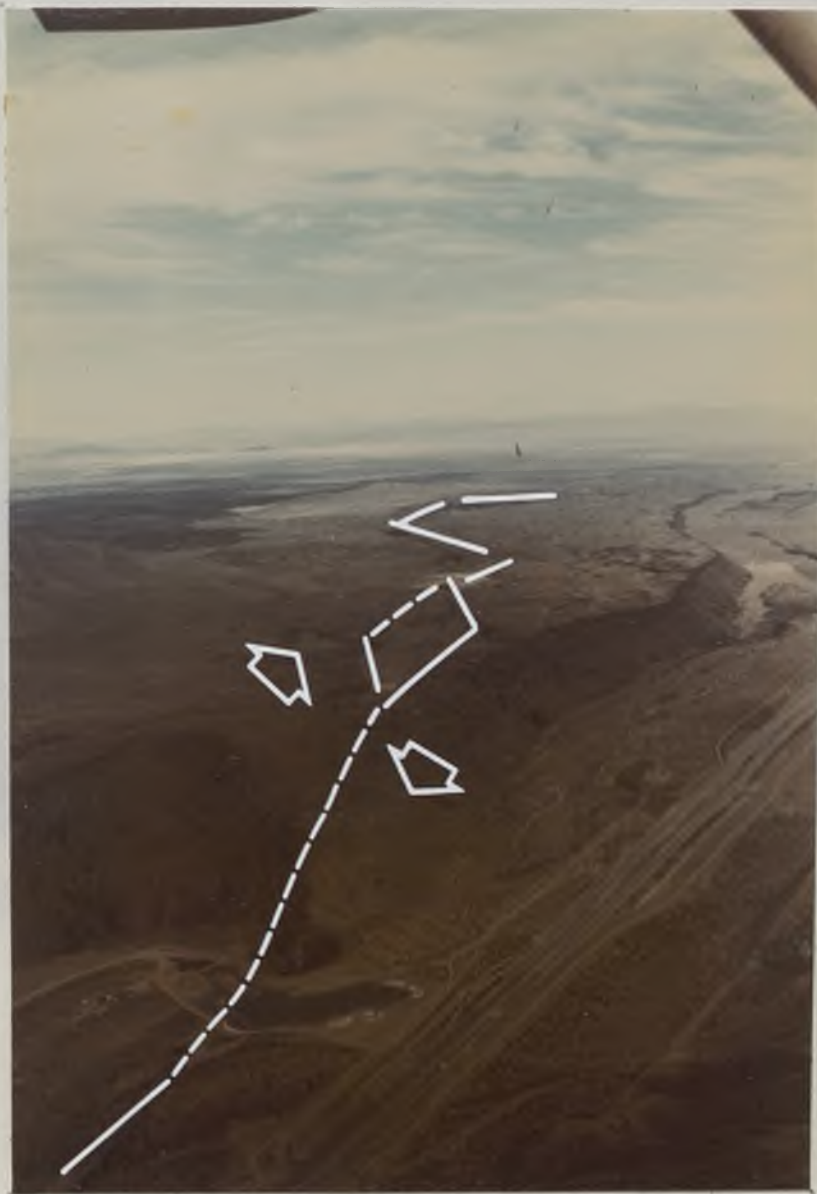
FIGURE 4. Aerial view of 250 meters of right-slip displacement caused by the Little Lake fault in a 400,000 year old lava flow.
