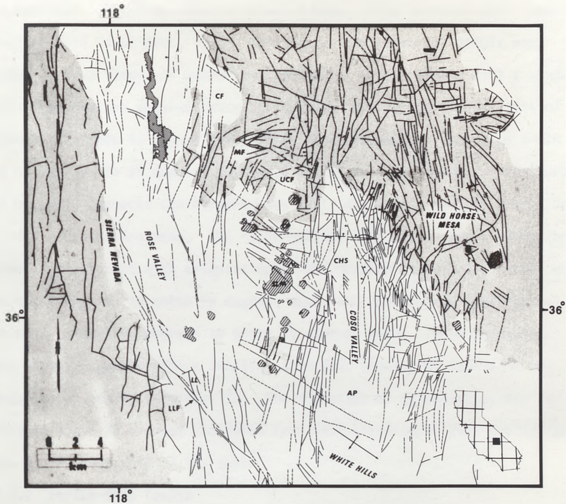
FIGURE 52. Fault map of the Coso Range. (AP) Airport Lake, (LLF) Little Lake fault, (LL) Little Lake, (SLM) Sugarloaf Mountain, (CHS) Coso Hot Springs, (CP) Cactus Peak, (UCF) Upper Cactus Flat, (MF) McCloud Flat, (CF) Cactus Flat. The shaded area marks the topography above 5000 feet. The hatched areas are rhyolite domes.
