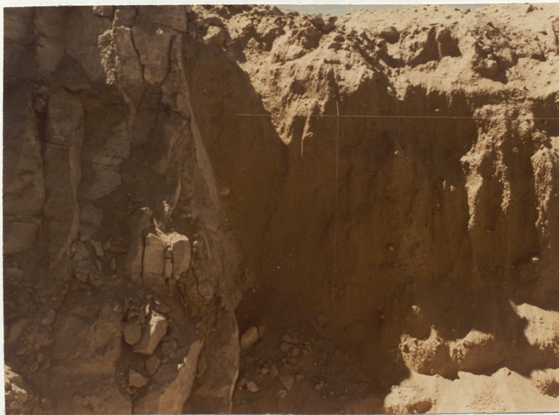
FIGURE 30. Slickensided fault plane in Trench B.
