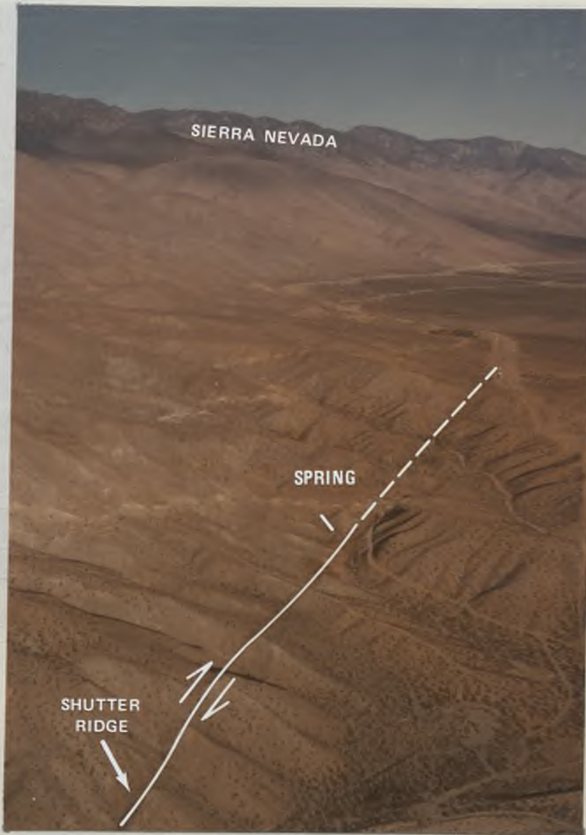
FIGURE 2. Aerial view of the Sierra front showing a shutter ridge caused by the Little Lake fault.
