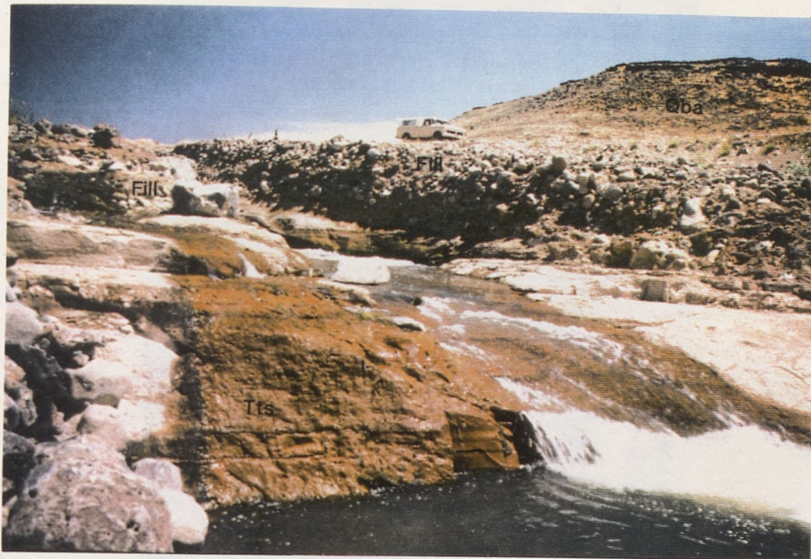
Figure 4. Photograph showing diatomaceous and tuffaceous sediments of the High Rock sequence (Tts) exposed in the Smoke Creek Reservoir spillway. Other units are dam embankment fill (Fill) and Quaternary basalts (Qba). View is toward the northeast.
